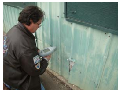
Testing for lead on the exterior
